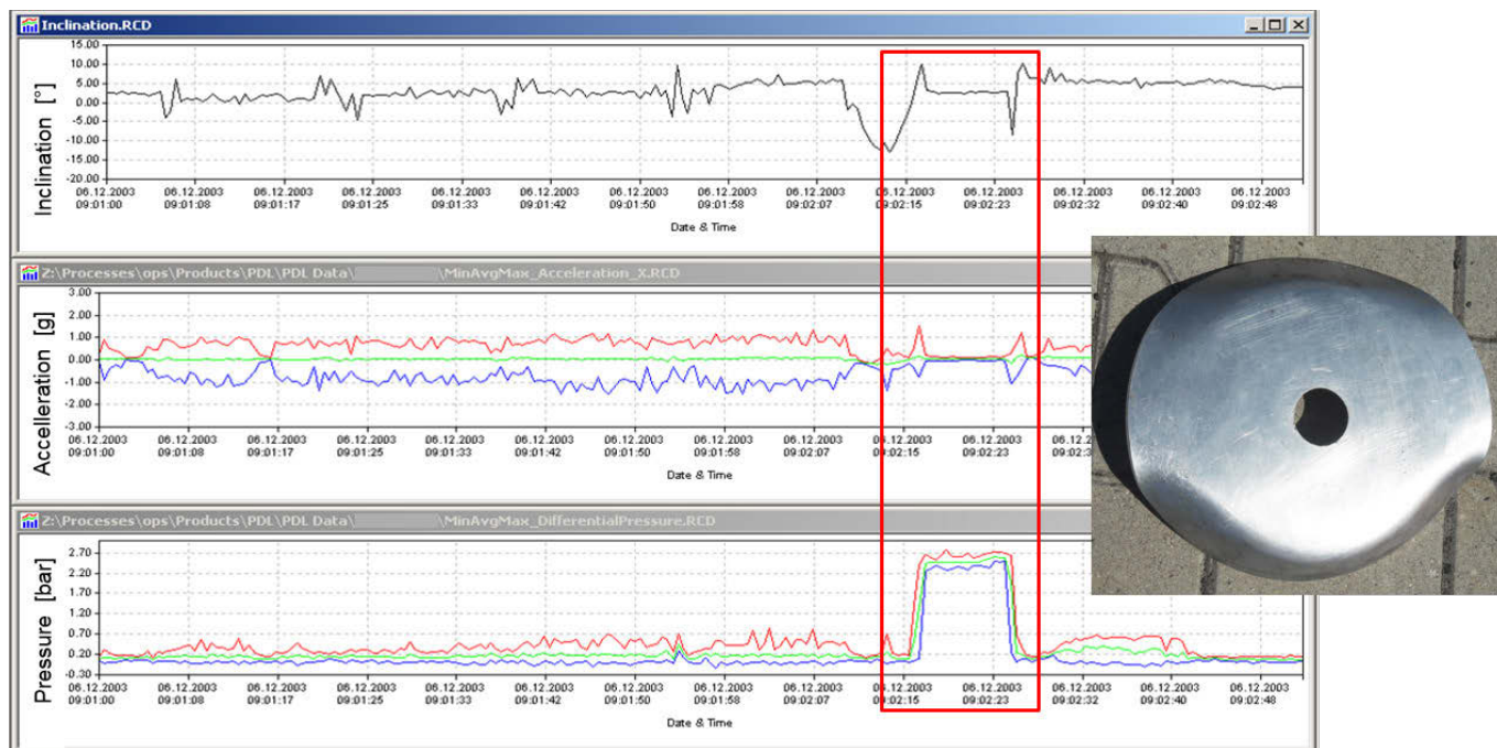
Figure 5: Cleaning tool PDL data analysis showing significant pipeline deformation led to a stuck tool. Buildup of pressure eventually dislodged the tool enabling run completion
