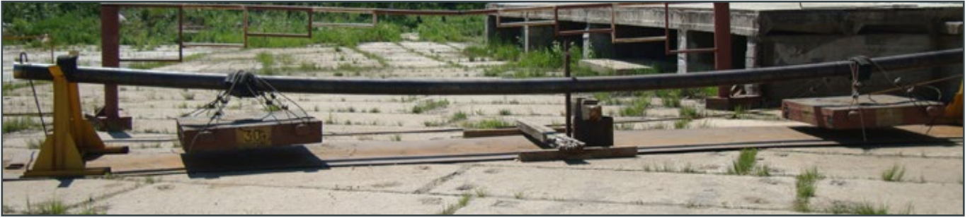
Figure 5: HFW combined load test (courtesy of JSC VSW (part of OMK))
