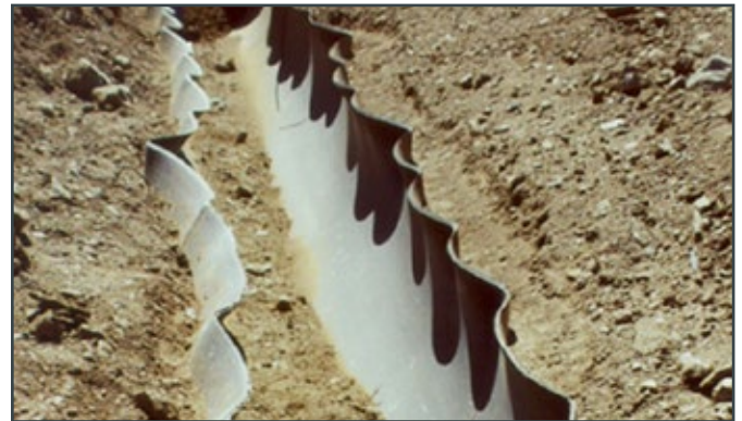
Figure 1: Example of ductile fracture propagation in a Rina test on a gas pipeline
