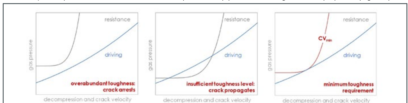
Figure 2: Illustration of the Battelle Two-Curve Model (BTCM) concept
