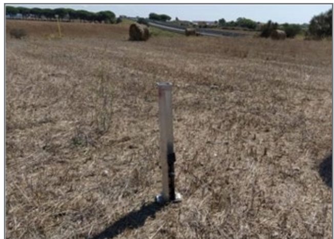
Figure 5: Calibrated weight-drop tool used to estimate the energy transference from the ground to the pipeline
